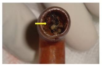
Fig. 2 Crusting within the T-tube.
